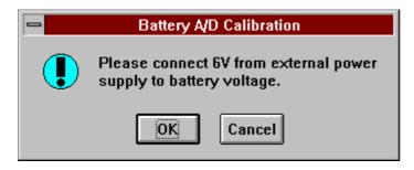
When an external power is connected, and the user selects OK to continue, the application measures a/d converter and displays the **Battery A/D Calibration** dialog box.
