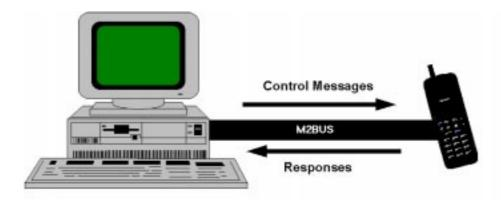
The recommended minimum hardware standard to run the Service Software package is any computer which is 386 33Mhz or greater with at least 4 MB of memory and VGA type display (640x480). This assumes that only the Service Software package is active, i.e. other Windows packages are not running in the background.
